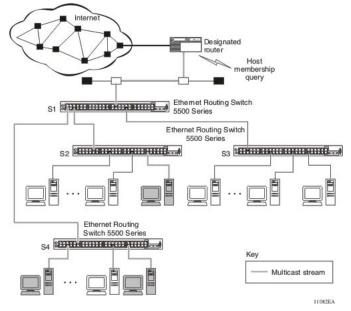
5500 Series switch filtering IP multicast streams (2 of 2)
